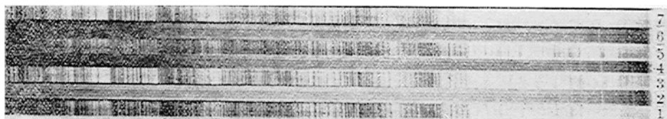
(1), (3), (5) and (7) Iron spectrum (2) Blank (4) Spectrum of the products at 10 mmHg. (6) The same at 5 mmHg.
